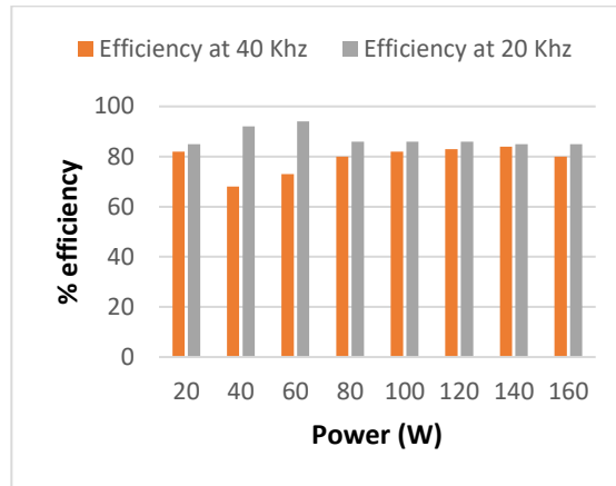
Fig. 8 Comparison of efficiency using synchronous rectifier at different operating frequencies
